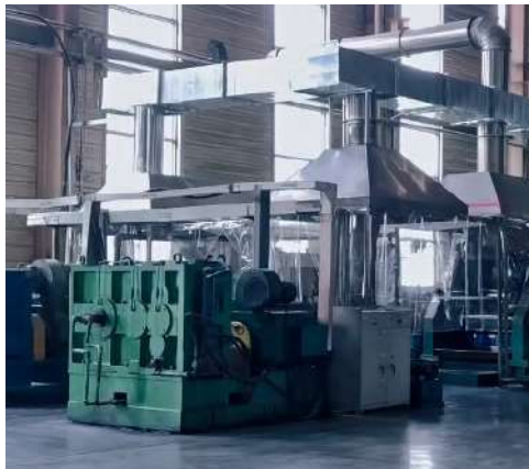
01 INNER TUBE EXTRUSION
