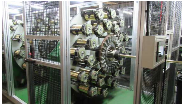
02A STEEL WIRE SPIRALING
